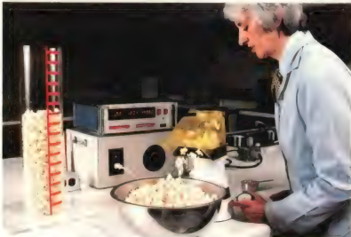
A researcher times how long it takes to pop corn and records how many kernels are left
